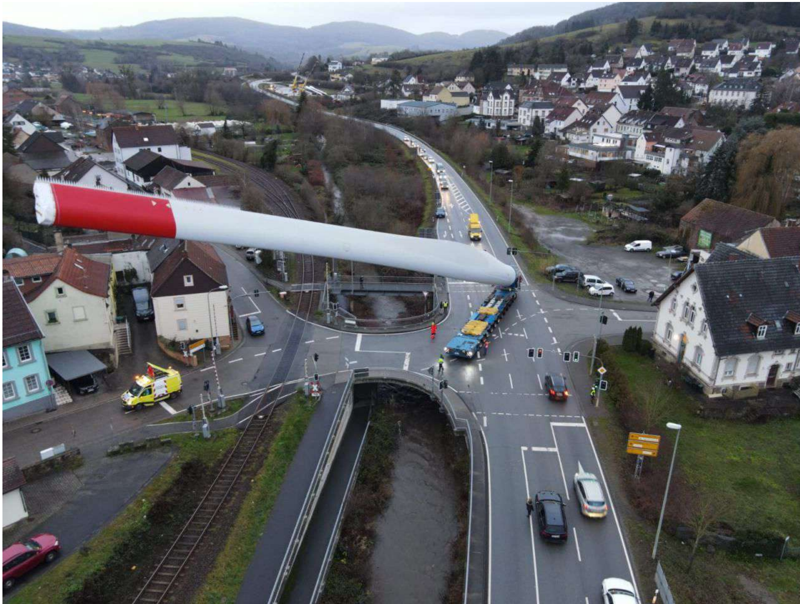
Source: P. Adams Schwertransporte, LinkedIn “Finishing the year with a set of 67m rotor blades on a challenging route”
